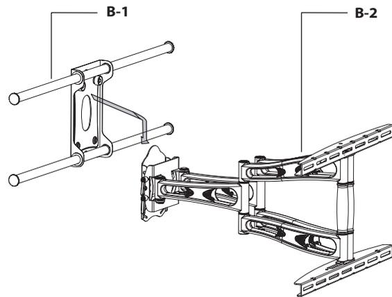
Attach part B-1 to part B-2 by hooking on.
