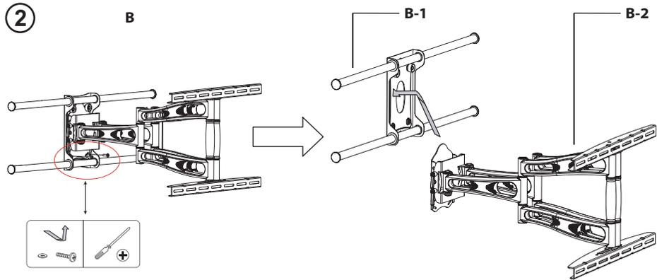
Use screw - driver to loose the screw, and divide B into B-1 and B-2.
