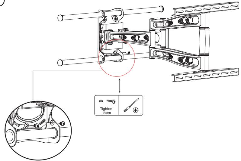
Tighten the screws as picture shows.
