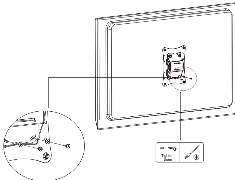
Tighten the screws as picture shows.
