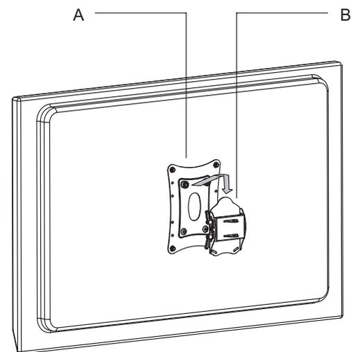
Attach part A to part B by hooking on.
