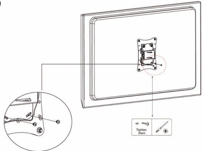
Tighten the screws as picture shows.
